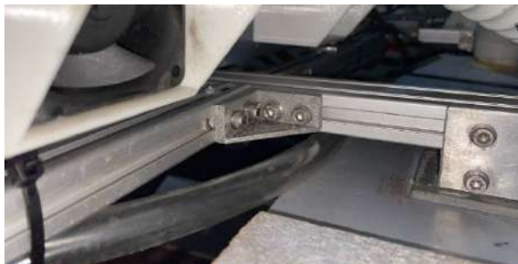
Fig. 15. Double slot angle bracket installation
